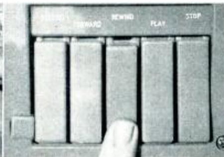
Five "piano keys" operate electro-solenoids which do the actual work of switching. Action on all movements is positive and rapid.
