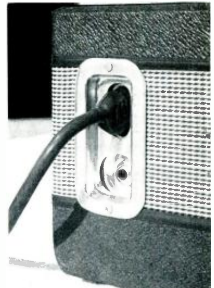
The power cord is plugged into the case as shown. Below this connection is the jack for use with an external speaker.
