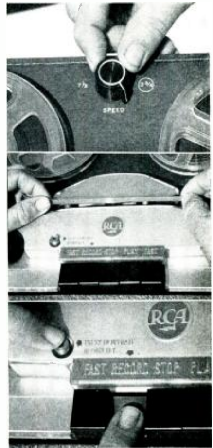
Top: change in speed is effected by turning knob to the desired speed, either 3\frac{3}{4} or 7\frac{1}{2} inches per second. The knob should not be operated while the machine is running. Center: to thread, the tape is dropped in the slot dull side away from the operator. By lightly depressing one of the other buttons, the stop button is released and threading made easier. Lower: to record, both the safety button and the record button must be depressed.
